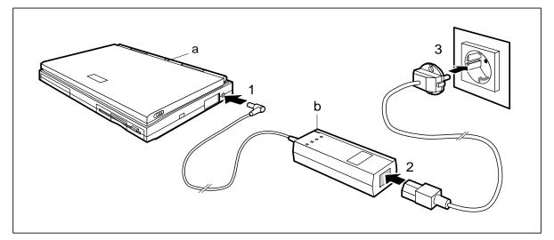
Plug the DC output connector on the power supply unit into the DC input connector on the notebook (1).
