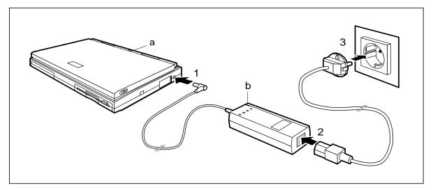
Plug the DC output connector on the power supply unit into the DC input connector on the notebook (1).
